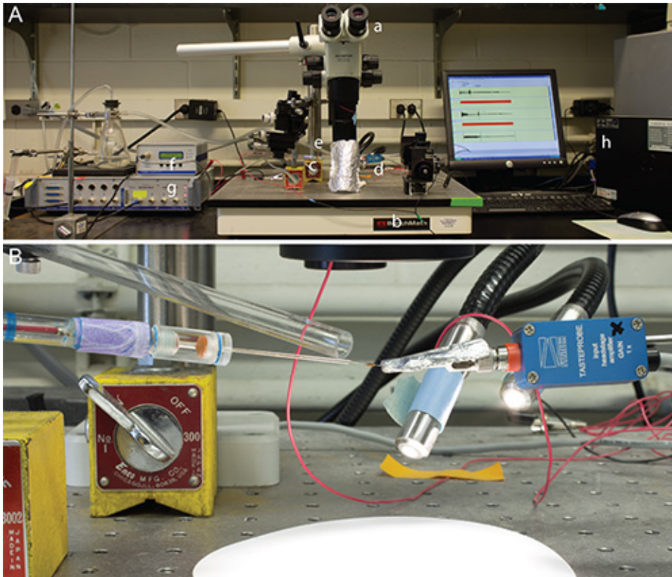
Figure 1. (A) Overview of recording rig setup. Stereomicroscope (a) is mounted on anti-vibration platform (b). Reference electrode holder (c) is mounted on platform opposite the headstage (d), via micromanipulators. An outlet plastic tube (e) delivering humidified air stream directed at the fly preparation is also mounted on the platform. The headstage is connected to the amplifier (f), which is connected to the digital acquisition system (DAS) (g), which is connected to a PC (h). (B) Configuration of electrodes and outlet tube: reference electrode on the left, recording electrode on the right, and air stream outlet tube directed at fly preparation. Click here to view larger image.
