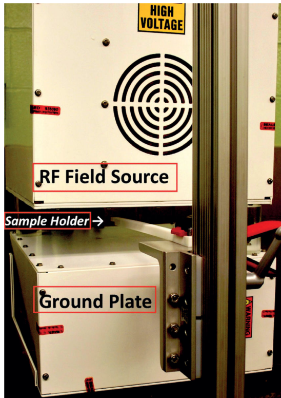
Figure 1. A radiofrequency field is created between the source plate (top) and the ground plate (bottom) when connected to an RF generator (not imaged)
