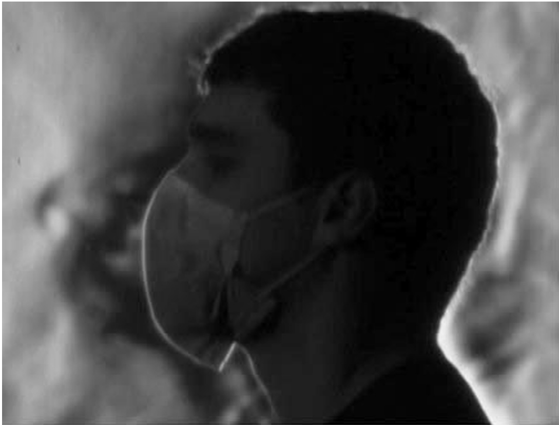
7 Schlieren optical imaging: Plumes of air from same individual as in Fig. 6 wearing PT mask. More air is exhaled through the mask with only a small amount of leak around the mask.
