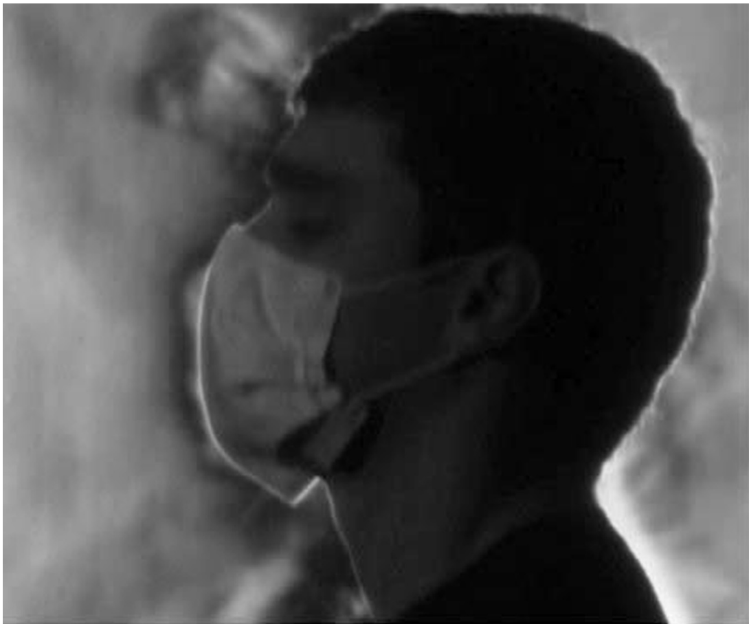
6 Schlieren optical imaging: Plumes of air during exhalation from healthy individual wearing SF mask, during tidal breathing. Air is leaking around the mask.
