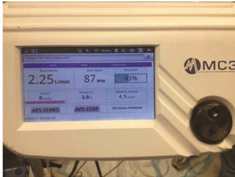
**Figure 3.** BioVAD console. The black dial in the lower right can be used to adjust the pump speed. The screen displays the pump speed in RPM, flow in liters per minute, amount of suction, and percent fill of the pump chamber.
