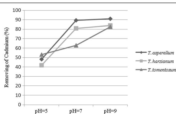
**Figure 1 Effect of pH on the removal ability of cadmium by *Trichoderma* species.** Maximum ability for cadmium removing was in pH = 9 for the all three *Trichoderma* species and the lowest removal ability was evaluated in pH = 5
