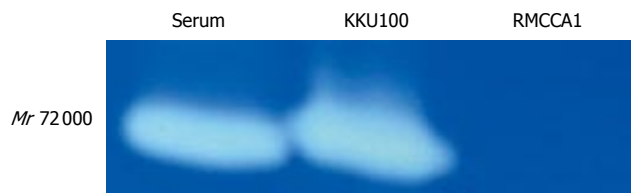
Figure 7 MMPs activity as determined by gelatin zymography. An intense band at Mr 72000 was shown in the FBS (fetal bovine serum) and the conditioned medium of KKU-100, but not of the RMCCA-1 cells. The Mr 72000 band in KKU-100 has previously been shown to correspond to MMP-2 activity in many cell lines [11,12] .
