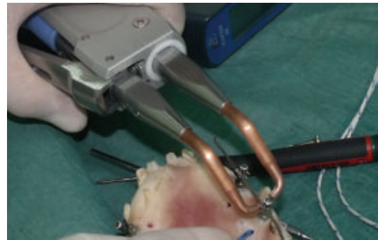
FIGURE 5: The resistance spot welding process.
