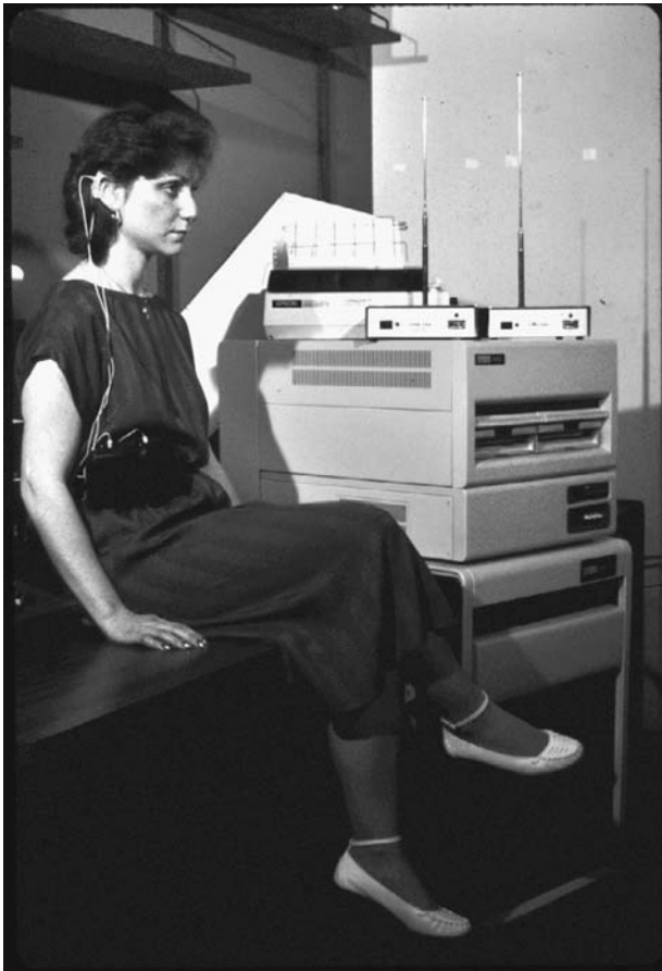
Figure 2. Photograph of the array processor digital hearing aid and a person using the system. Photograph reprinted with permission of the City University of New York.
