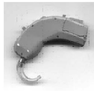
Figure 4. Photograph of the Project Phoenix behind-the-ear digital hearing aid. Photograph reprinted with permission of Audible-Difference®.
