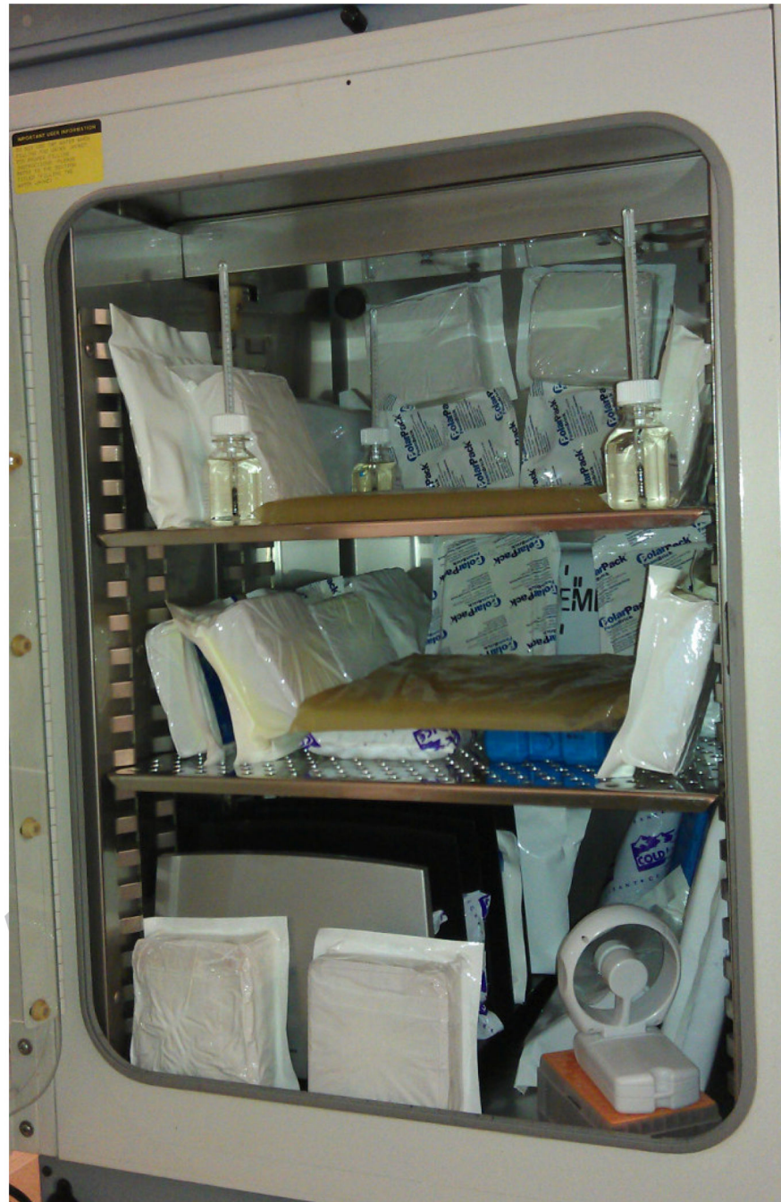
Figure 3. Incubator set up for heat shock experiments. The image below shows our efforts to get as much warm surface area as possible into the incubator. Shown is a Forma Scientific water-jacketed, stacked incubator, model 3327. The top shelf was chosen for the experimental space because, without the fan running, it was the shelf that most frequently stayed at the temperature set on the incubator. The middle shelf tended to be lower than desired and the bottom shelf lower still. Although this was less than a 1°C difference from top to bottom, that can be enough to affect the outcome of an experiment. The bottom shelf has a desktop
