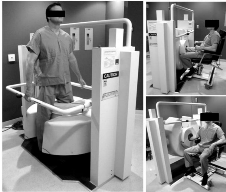
Figure 1. The extremity CBCT unit currently in clinical pilot studies in a standing configuration for imaging of weight-bearing lower extremities in natural stance and in a sitting configuration for imaging of lower and upper extremities
