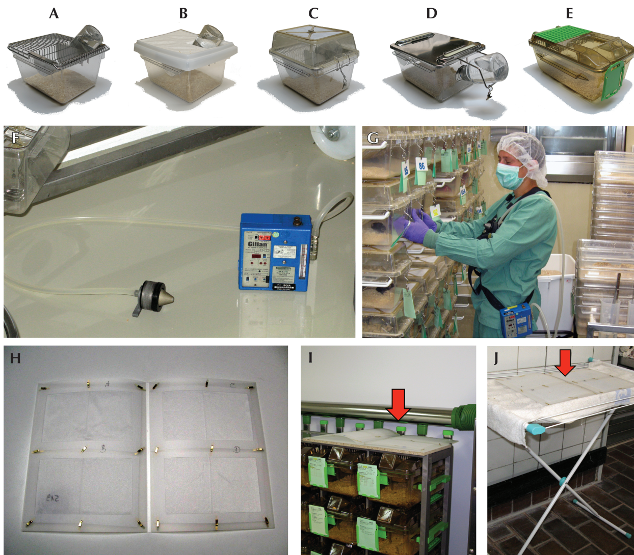
Figure 1. Cage types and sampling methods. (A) Type II open polycarbonate cage (floor area, 344 cm 2 ; height, 13.5 cm) with wire lid holding chow and water bottle. (B) Same cage setup as in panel A but with an additional soft filter top composed of a flexible polyethylene frame holding a polypropylene filter. The water bottle is positioned halfway across the cage, through a cross cut in the paper filter of the filter top. (C) Same cage setup as in panel A but with an additional rigid filter top composed of a rigid polycarbonate frame holding a polyester filter (static microisolation caging). (D) Same cage set up as in panel A but covered with a nonsealed, solid stainless-steel lid and used in an IVC rack as described. The cages shown in panels A through D had no seal between cages and lids. (E) Type II long, sealed, polyphenylsulfone cage (floor area, 501cm 2 ; height, 13.5 cm) with polyphenylsulfone lid holding a polytetrafluorethylene membrane filter and used in an IVC rack. Silicone gaskets were placed between cages and lids. (F) Stationary air pump and sampling head carrying a filter for the collection of ambient samples. (G) Portable air pump with sampling head attached to a staff member for the collection of samples from the breathing zone at the upper chest level during cage changing on a stainless steel table. (H) Electrostatic dust fall collectors (EDC) for the collection of ambient samples. (I) EDC (arrow) positioned on top of an IVC rack. (J) 2 EDC positioned on a sampling table in the wash room.
