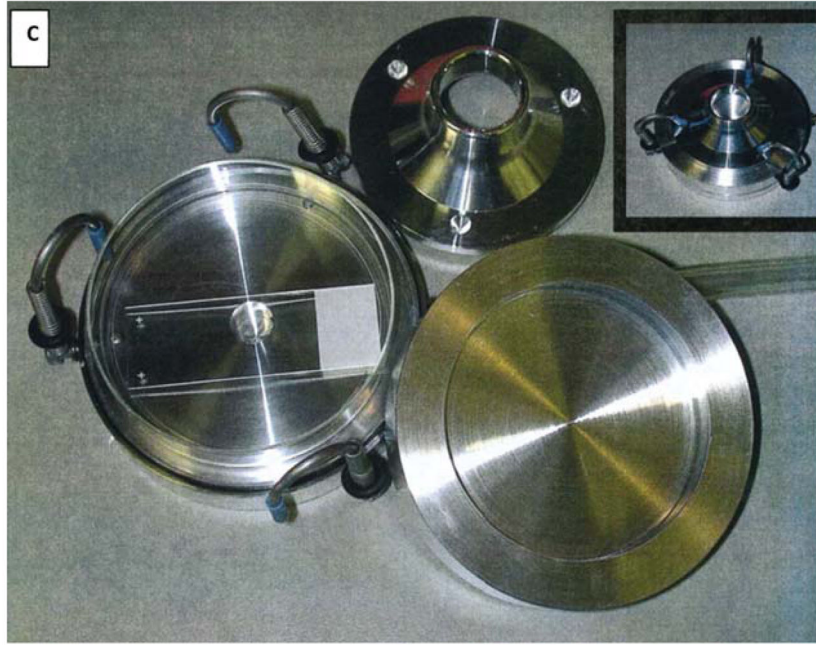
Figure C. Disassembled impactor showing slide placed inside Petri dish. See http://www.skincinc.com/prod/225-9611.asp )
