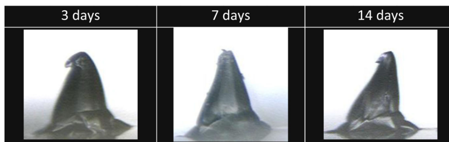
Figure 10. Percentage reduction in the height of microneedle arrays under an axial load of 0.2 N per needle after storing at 0% RH and 43% RH for different time intervals (means \pm SD, N = 6) (A) and representative digital microscope images of microneedles stored at 86% RH (B).
