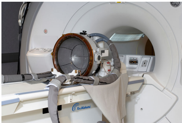
Fig. 1 Magnetic resonance-guided focused ultrasound transducer helmet on a magnetic resonance imaging table. The model shown is ExAblate Neuro (InSightec, Haifa, Israel). The hose to the helmet carries cooled, degassed water that will provide the medium through which acoustic energy passes
