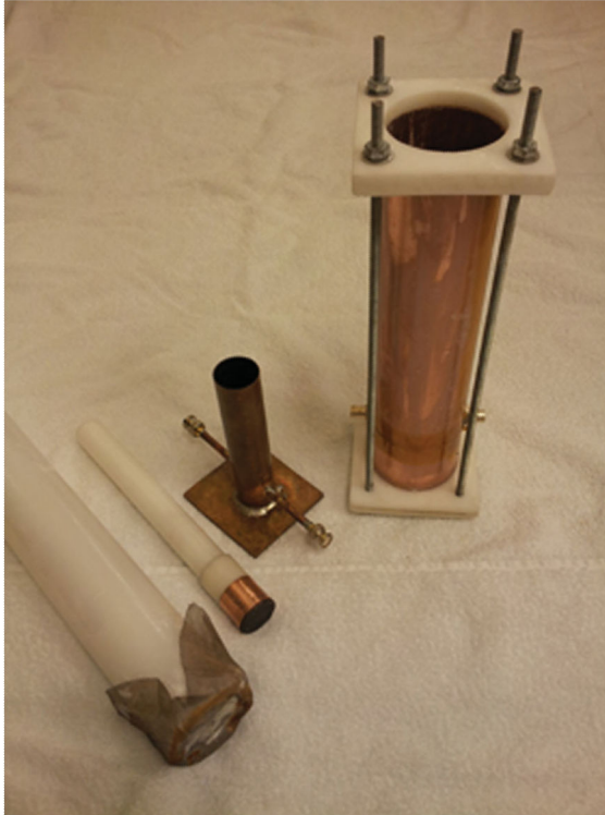
FIG. 1. Resonant cavities used to characterize the BaTiO 3 bead slurry. [Color figure can be viewed in the online issue, which is available at wileyonlinelibrary.com .]
