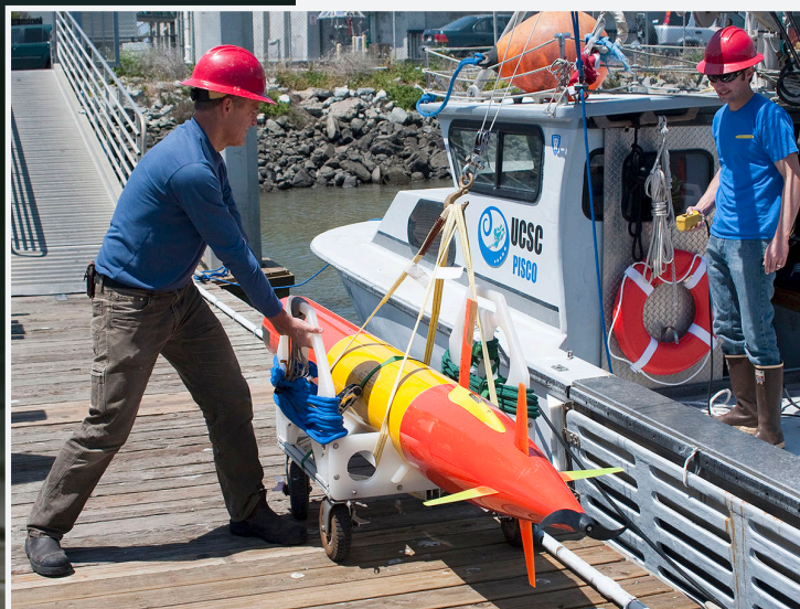
In a mooring configuration developed at Woods Hole Oceanographic Institution, the second-generation Environmental Sample Processor, or ESP (left), automatically collects and tests water samples for DNA and toxins that indicate the presence of HABs. A much smaller third-generation ESP mounted within a long-range autonomous underwater vehicle (above) will be able to physically follow and monitor developing blooms. The new ESP should be commercially available within three to four years. Schematic: © E. Paul Oberlander/WHOI; photo: © Todd Walsh/MBARI
