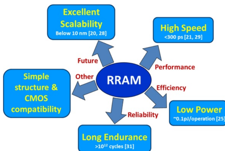
Figure 1 Prospective of RRAM devices. Endurance, speed, scalability, and requirements of RRAM devices.
