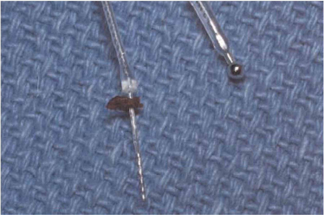
Figure 1. Nucleus Hybrid S8 electrode with a small piece of fascia abutting the Dacron collar (left); ground electrode (right).
