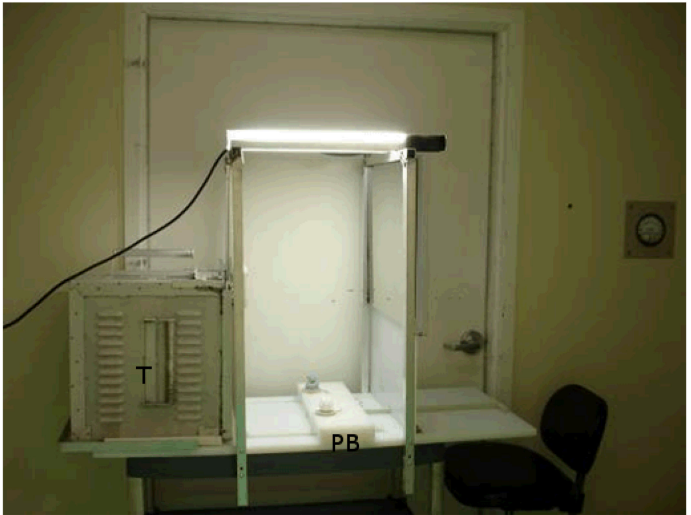
Figure 2. Photograph of a WGTA testing station. The transfer cage is labeled T and presentation board as PB, with a blue and white toy as the stimulus objects covering the wells for reward placement.
