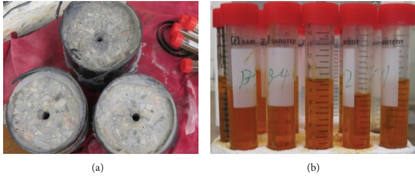
FIGURE 7: Ponding test: (a) concrete specimen with NaCl solution on top; (b) mixing concrete powder with NaCl solution.
