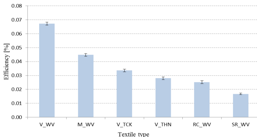
Fig. 7. Efficiency of light coupling into photonic textile with its standard deviation (n = 5)
