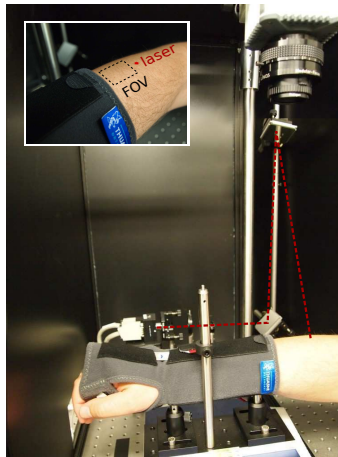
Fig. 3. The photograph of the setup for the in vivo experiment. The inset figure depicts the approximate location of the source and the field-of-view.
