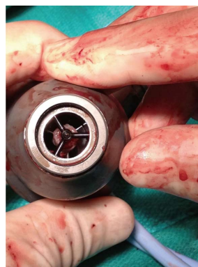
Figure 2 Inspection of the pump revealed a firm thrombus along the inlet stator.
