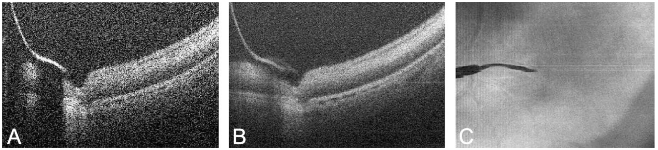
Fig. 3. Microscope-mounted OCT image of 36-gauge retinal needle with cadaveric porcine retina. A. Single B-scan of retinal needle showing high reflectance at area of needle with absolute shadowing of underlying tissue. B. Summed B-scan series of retinal needle showing improved tissue visualization and significant improvement in shadowing. C. Summed voxel projection of retinal needle on retinal surface.
