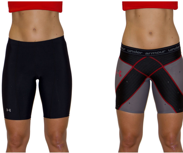
Figure 1. Participant wearing traditional compression shorts which stretch isotropically in all 4 directions (left), and directional compression shorts (right) with diagonal bands of fabric that only stretch along their length (black fabric). The same sizing guidelines were used to fit both types of shorts to each participant.
