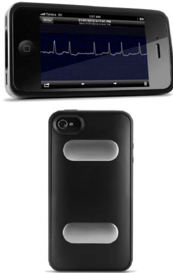
Figure 1. Alive Cor real-time monitoring of ECG. Finger contact on the case activates ECG recording of bipolar lead I and is transmitted to the smart phone.
