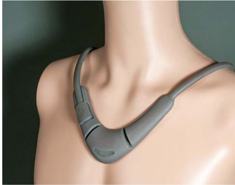
Figure 4. Perminova CoVa necklace uses thoracic bioimpedance and ECG monitoring to determine stroke volume, blood pressure and cardiac output in patients with chronic cardiac conditions.
