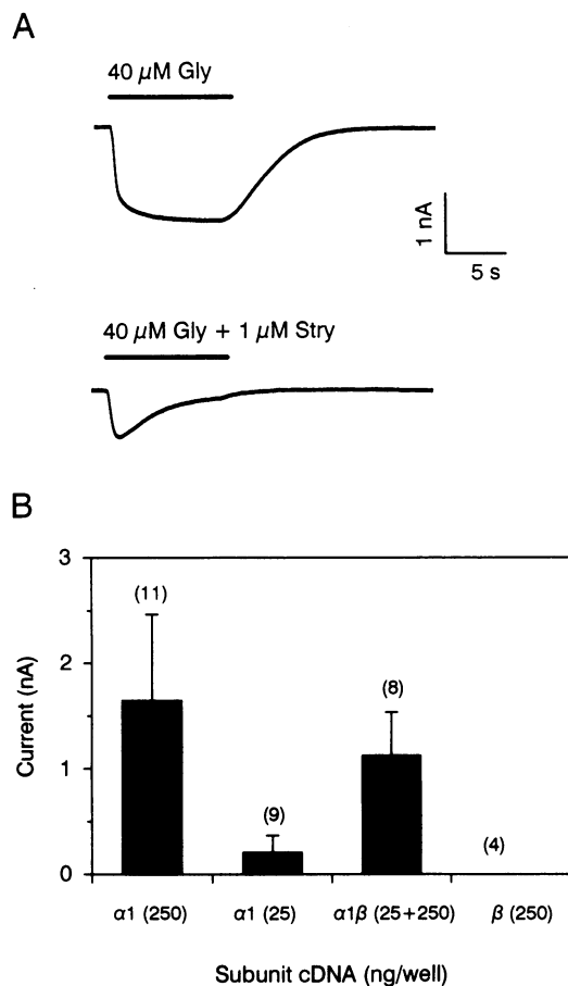
Fig. 1. Functional expression of homo- and hetero-oligomeric GlyRs in HEK-293 cells. (A) Whole-cell current induced in cells transfected with 250 ng \alpha 1 cDNA. Application of 40 \mu\text{M} glycine (Gly) gives rise to an inward current, which results from the outwardly directed movement of \text{Cl}^- ions (top). The cell was recorded with intra- and extracellular \text{Cl}^- of 145 mM and clamped at -70 mV holding potential. Upon co-application of 1 \mu\text{M} strychnine (Stry), the glycine response showed an initial peak, which rapidly declined to almost baseline level (bottom). (B) Co-expression of \alpha and \beta subunits. Cells were transfected with various amounts of \alpha 1 and \beta cDNAs. Numbers denote ng cDNA/cover slip. Average whole-cell currents induced by 40 \mu\text{M} glycine are plotted ( \pm SD) on the ordinate. In cells transfected with \alpha 1 alone, the current strongly depended on the cDNA dose. With \beta cDNA alone, no measurable response was recorded. Upon co-expression of a low dose of \alpha 1 (25 ng) plus a 10-fold excess of \beta cDNA, currents were markedly elevated as compared to the average response obtained with 25 ng \alpha 1 cDNA alone.
