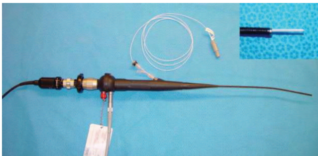
FIG. 1. Flexible endoscope with inserted magnetic tracker. The inset in the upper right corner shows the 1.3 mm diameter sensor slightly protruding from the working channel of the endoscope.
