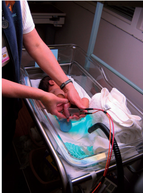
Figure 1. Photograph of an infant's skin carotenoid measurement via Resonance Raman spectroscopy, RRS. The instrument's fiber-coupled light delivery and collection module is held against the foot, exposing the heel skin to weak 488 nm laser light for 20 seconds. From spectral analysis of the Raman scattered light intensities, which occur in the green wavelength region, the carotenoid levels in the heel skin are obtained in a rapid, non-invasive, and painless fashion.
