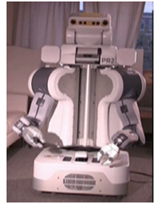
Fig. 1 A screenshot of the Willow Garage's mobile manipulator, the Personal Robot 2 (PR2), as shown in a video to participants
