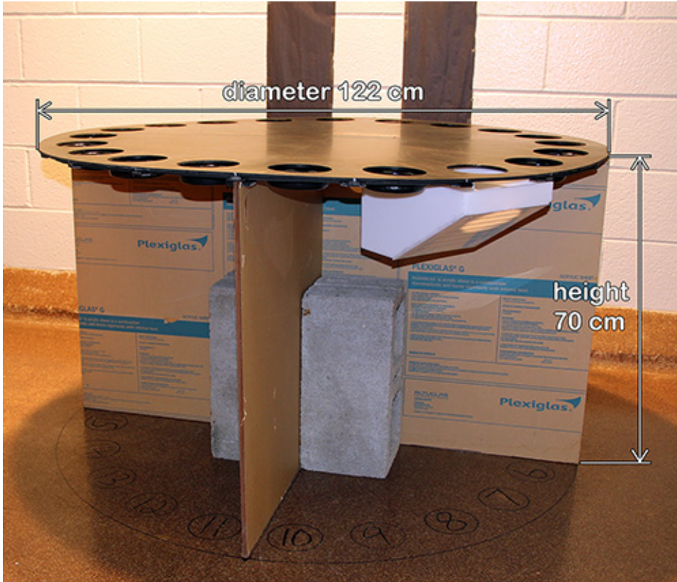
Figure 2. The Barnes maze apparatus for rats. The maze top and supporting stands can be seen with maze top diameter and height from floor shown. Numbers on the floor indicate hole numbers and allow the tester to place the escape cage in the designated location (the floor numbers cannot be seen by the subject). One of the extra-maze visual cues can be seen on the far wall (i.e. black vertical stripes). Click here to view larger image.
