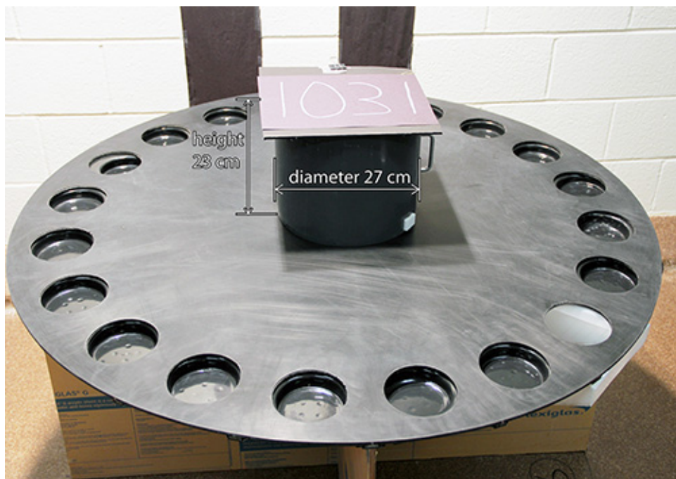
Figure 4. The center tube with sample subject identifying sheet on the top of the Barnes maze apparatus for rats. The cardboard cover lifts away to place the rat inside the tube and is then replaced. The handle on the center tube allows easy lifting to begin the trial. Click here to view larger image.
