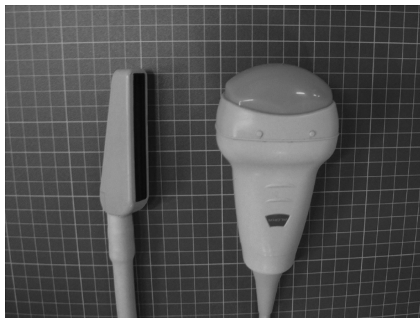
Fig. 1. Appearance of transducers. The convex transducer is able to image at up to 30 cm depth and can readily be operated in mare's rectum, because of its form.
