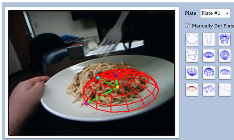
Fig. 3 (colour online) Part of the software interface for portion size estimation. The wire frame in the picture represents the selected shape model and the four dots represent the control points that can be dragged to adjust the size and location of the model. The right part of the menu shows the shape model library
