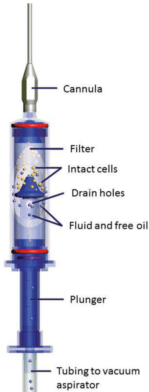
Figure 1. Schematic of the LipiVage Device. The LipiVage device was designed to harvest small volumes of autologous adipose tissue for cosmetic surgical applications. The device aspirates fat at low vacuum into a sterile chamber. Once inside, the fat cells are concentrated by filtration. Fluids and free oil are drawn into a waste canister. Diagram courtesy of Genesis Biosystems
