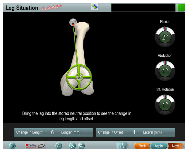
Fig. 2 In the navigation group, intraoperative leg length and offset changes were calculated by the navigation system and shown on the screen. Int. rotation = internal rotation.
