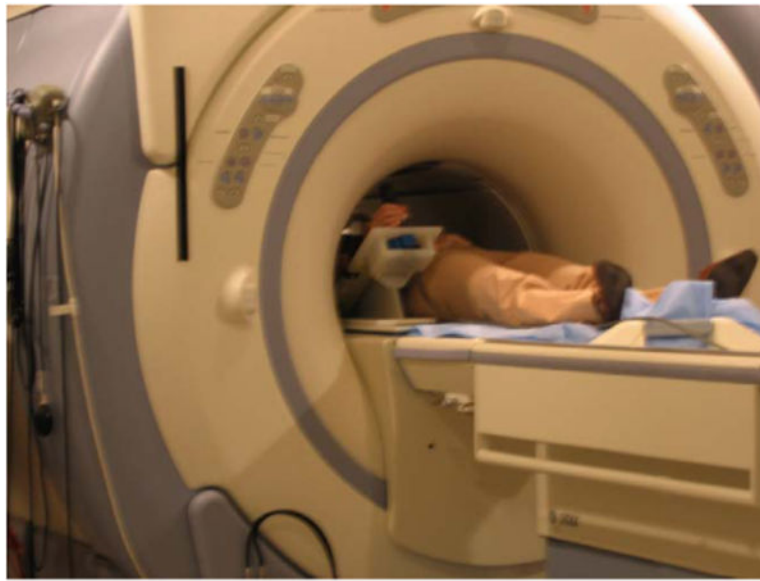
Fig. 5. Illustration of the wrist device being used inside the scanner during fMRI testing. The wrist module is normally located just inside the scanner bore, dependent on the size of the test subject.
