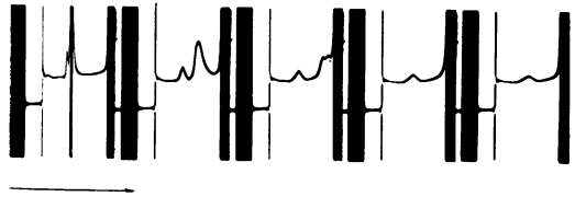
FIG. 6. Ultracentrifugal pattern of phenol extract I from H. capsulatum (intact cells). The extract (10 mg/ml) was dissolved in 0.015 M Tris buffer (pH 7.75) and sedimented at 59,780 rev/min (259,700 \times g) at 20 C in a synthetic boundary cell. Photographs were taken at 16-min intervals starting at 0 time.
