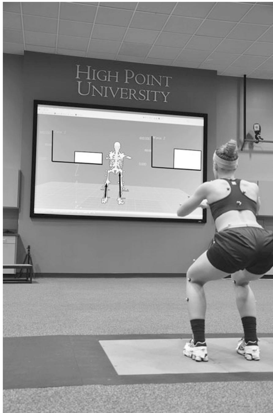
Fig. 2. Real-time feedback during a squat. The patient receives information on the magnitude and direction of ground reaction forces. Visual and auditory cues are provided to correct imbalances
