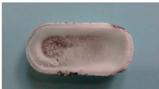
Figure 1. Nanostructures visible as a white fluffy mass with naked eyes formed at the edges and the top of the quartz boat.
