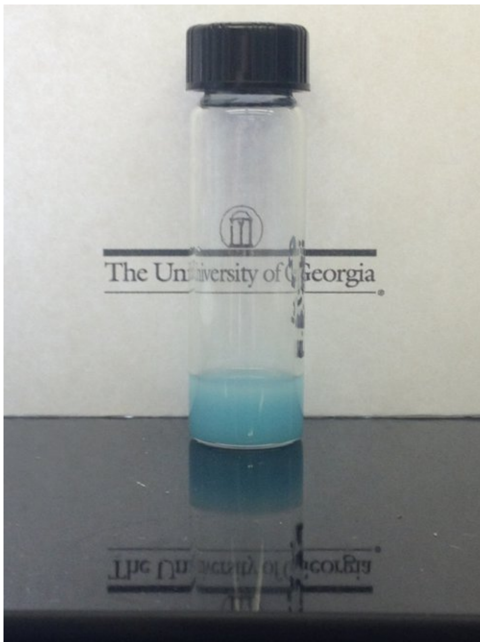
Figure 9. Photograph of a \text{CaCuSi}_4\text{O}_{10} nanosheet ink in a vial.
