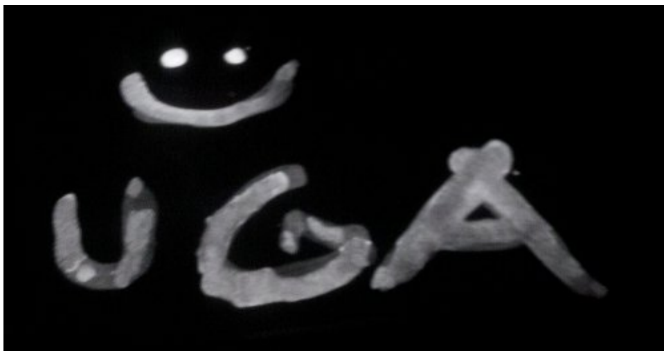
Figure 10. Near Infrared Imaging. A rudimentary painting with the \text{CaCuSi}_4\text{O}_{10} nanosheet ink that illustrates both its simple application and its luminescence properties.
