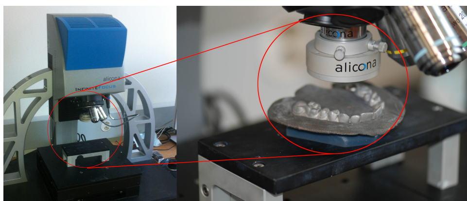
Figure 17: Preparing a full arch model scan. A) Scanning without the base B) Repeatability at the model margins is low because of the high angulation of the tooth surface, especially in the anterior region C) The superimposition of different scanning directions shows a deformation of the scan, starting in the anterior region of the model D) Applying a horizontal base around the model with a material of equal light reflection properties E) Scanned model and base show high repeatability all around the scan object F) The superimposition of different scan directions shows only small local deviations but no entire deformation of the scan. Click here to view larger image.
