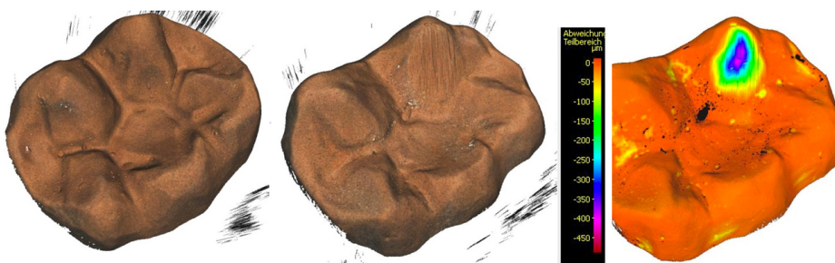
Figure 21: Difference image between a test specimen before and after chewing simulation, color graded from -20 µm (orange) to -500 µm (purple). The high-resolution scan of the tooth surface is used to evaluate the abrasion of different restorative materials with in vivo and in vitro tests. Click here to view larger image.
