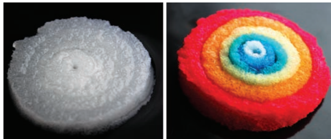
Assembly of six concentric “donuts” of silk scaffold, original color (Left); dyed with food color (Right).
