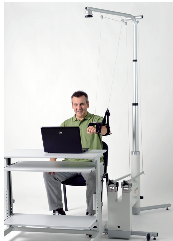
Figure 3. Armeo® Boom: a simplified cable-driven manipulator designed for out-patient clinics and home settings (reprint with permission by Hocoma, Swiss Federal Institute of Technology, Zurich - Switzerland).
