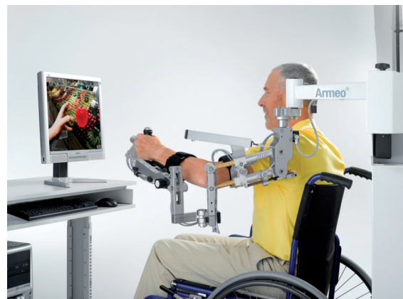
Figure 2. Armeo® Spring: an ergonomic arm exoskeleton with integrated springs (reprint with permission by Hocoma, Swiss Federal Institute of Technology, Zurich - Switzerland).
