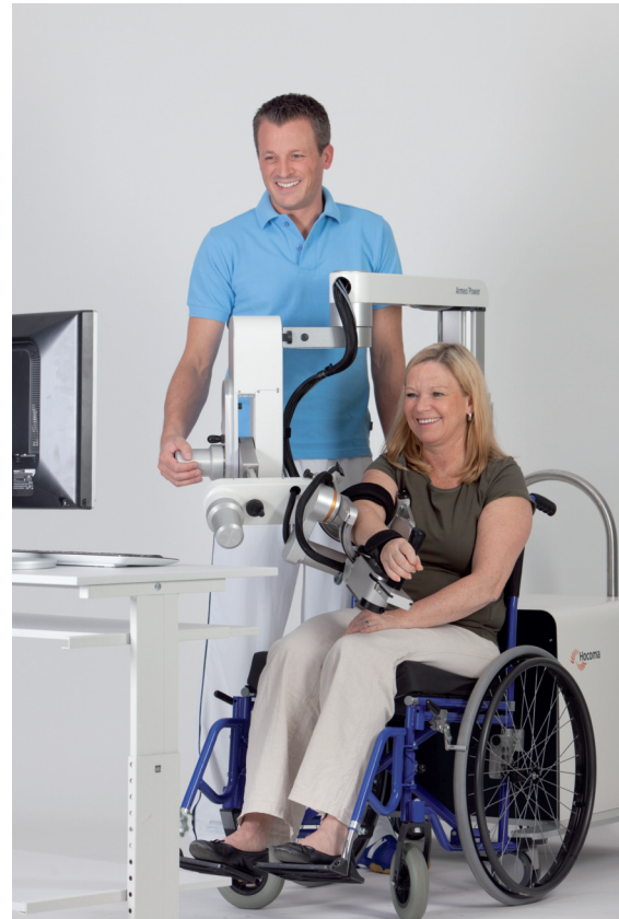
Figure 1. Armeo® Power: an exoskeleton based on the ARMin technology (reprint with permission by Hocoma, Swiss Federal Institute of Technology, Zurich - Switzerland).
