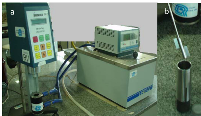
Fig. 1 Brookfield rotary viscometer (a) and small sample adaptor with flag impeller spindle (b) employed for evaluating the cooking profile of the starch samples
