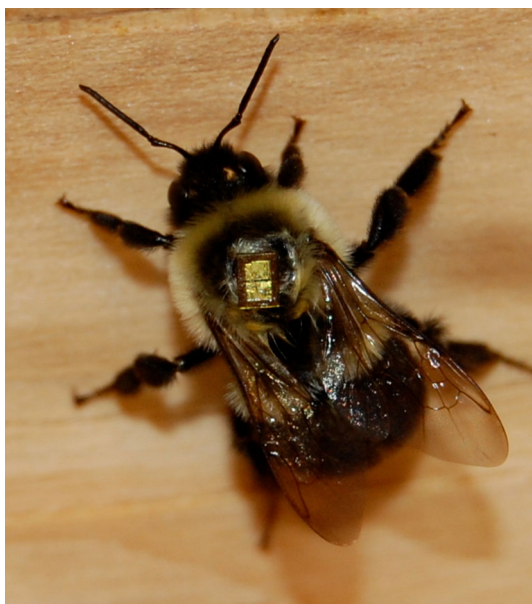
Fig. 2 B. impatiens worker tagged with RFID chip. © L.L. Orbán
