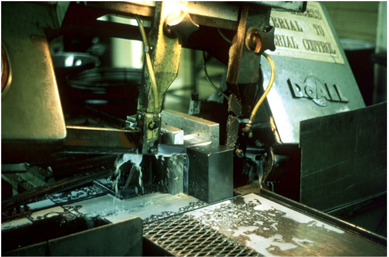
Figure 1. METALWORKING FLUID EXPOSURES CAN CAUSE SARCOIDOSIS-LIKE ILLNESS IN METAL MACHINING INDUSTRIES. Metal parts are commonly flooded with synthetic and semi-synthetic oils that serve as coolants during machining. Such fluids are commonly recycled and can become contaminated with mycobacteria, endotoxin, and microbial antigens. Workers often develop hypersensitivity pneumonitis that is initially mistaken for sarcoidosis.
