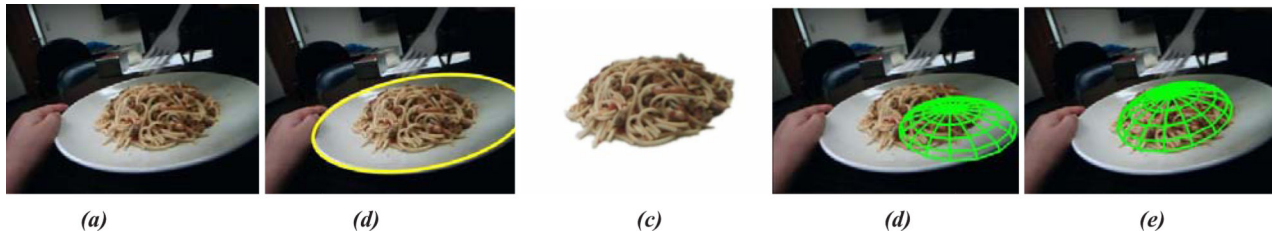
Fig. 3. Food image processing: (a) raw image, (b) dining plate detection, (c) food segmentation, (d) food shape modeling, (e) fitting result
