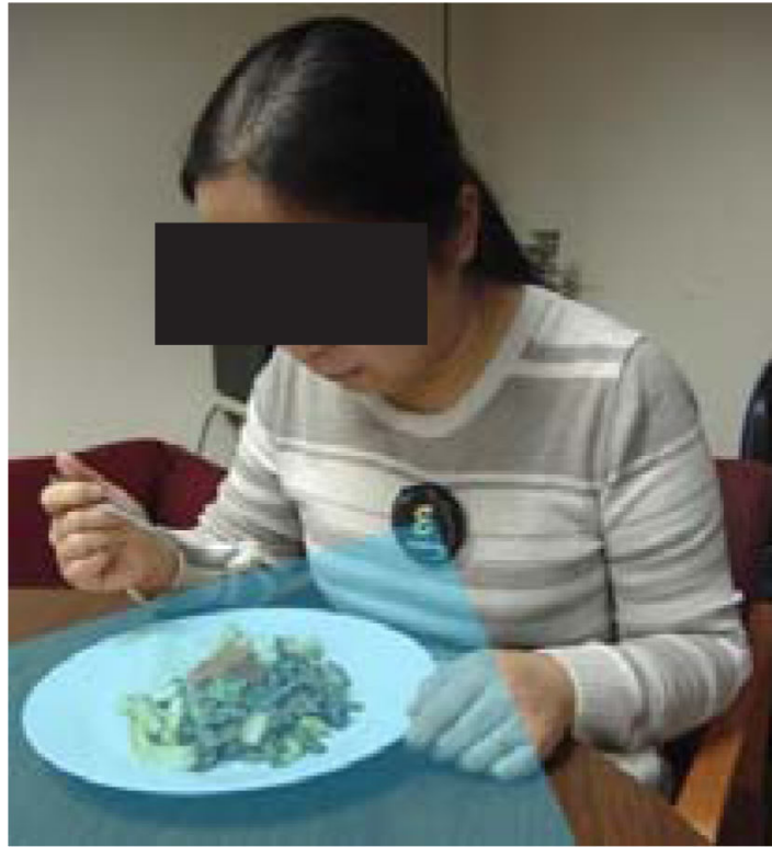
Fig. 2. The cameras on the eButton automatically take pictures of food
