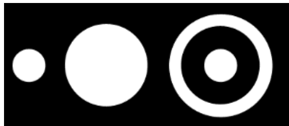
Fig. 1. Pupils for which monocular through-focus visual acuity was measured: a 1.6 mm pupil, a 4 mm pupil, and a 5 mm pupil with obscuring annulus (inner inlay diameter 1.6 mm, outer inlay diameter 3.8 mm).
