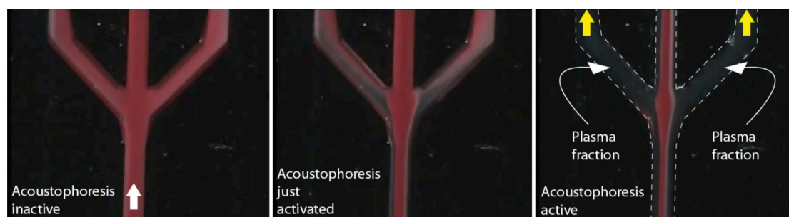
Figure 4. Sequence showing the starting phase of plasma production where A) ultrasound is inactive, B) the acoustophoresis is beginning to focus the RBC in the channel centre and C) continuous phase of plasma production where the final fraction of RBC are removed via the central outlet.
