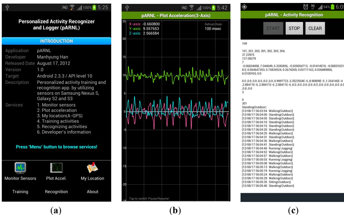
Figure 6. Smartphone application which implements real-time activity recognition framework. (a) Initial state of application. Sensor monitoring, accelerometer visualization, UI for activity training & recognition; (b) Visualizing 3-axis accelerometer values of walking activity; (c) Screenshot of activity recognition results.
